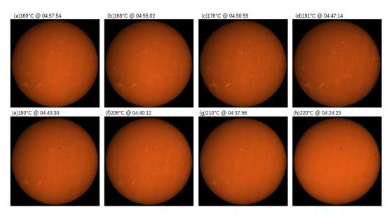
**Fig. 10.** Observing the lower solar atmosphere by a tuneable sodium MOF application on 30 July 2013, showing the solar intensity. The temperature of the MOF varied from 160 °C to 220 °C. UTC time and temperature values for each panel are labeled on the snapshots individually. The sequence of images outlines an intensity map scan descending from the mid-chromosphere downward toward the photosphere.
