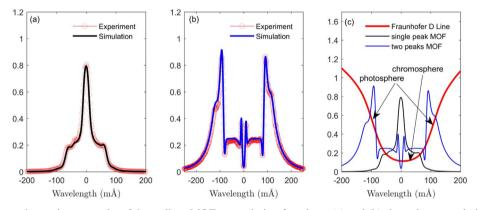
**Fig. 8.** The simulation and experiment results of the sodium MOF transmission functions. (a) and (b) show the transmission functions of Na D MOF with a center peak and with two wing peaks, respectively. Panel (c) shows the sodium MOF filter that has a single peak in the Fraunhofer D2 line center, enabling chromospheric filtering. The red solid line is the Fraunhofer line and the blue and black solid line are the MOF transmission functions.
