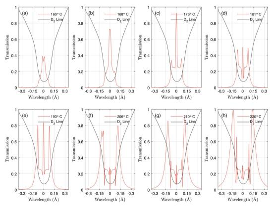
**Fig. 11.** Simulation results of transmission function for the sodium MOF. The temperature of MOF is changed from 160 °C to 220 °C. The magnetic field is 200 mT, and the length of cell is 25 mm. The Na  $D_2$  line is from (Wallace et al., 2011).
