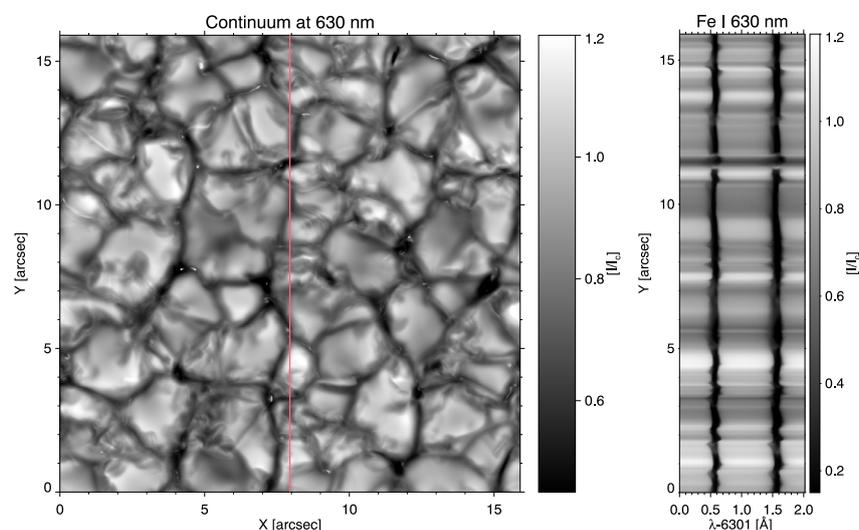
Figure 1. Left panel shows the continuum intensity at 630 nm. Red vertical line displays a reference slit position. Rightmost panel shows the Fe I 630.1 and 630.2 nm spectral lines for the reference slit. Image credit: Silvia Regalado Olivares (IAC).
