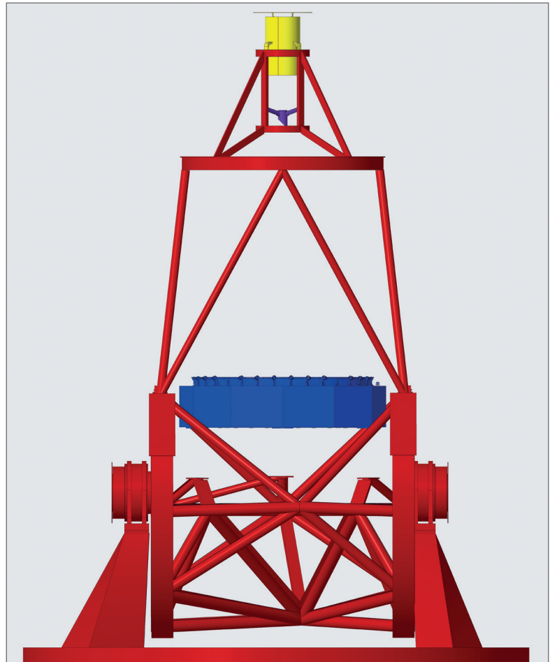
Figure 1. Telescope structure. The primary and secondary mirrors are in blue and yellow
